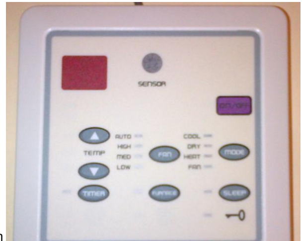
Wall mounted Thermostat control. An AC only model (AC-1361) will not have the furnace pushbutton on the wall pad unit.
