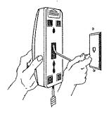
Connect coiled end of cord to Handset and, then, plug straight end of cord in wall phone modular jack.
