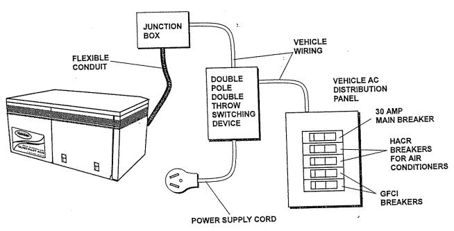
Figure 2.13 - Installation With Isolation Receptacle
