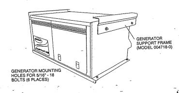
The installer must make certain that the selected of location will permit adequate cooling and ventilating airflow to be supplied.
