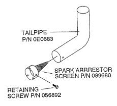
Figure 2.12 — Spark Arrestor Installation
