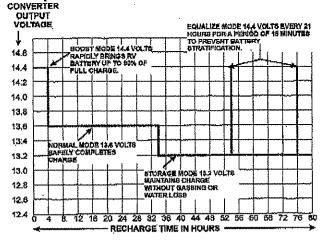
The chart below shows the amount of time it took a converter set to three different output voltages to recharge a 125AH (Amp Hour) battery after it was discharged to 10.5 volts.
