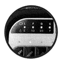
By pressing and holding the desired tank button for three seconds, the user receives a continuous readout
